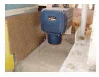
MoistTech's NIR moisture sensors are easy to set-up and use which will provide instant and precise measurements due to no constituent losses in handling. We recommend installing sensor(s) in several locations though out the process. A sensor should be installed over the conveyor before the final crusher to enable elimination of impurities, as well as at the exit of the final crusher or dryer, to prevent over drying and dust. The sensor should be installed several
