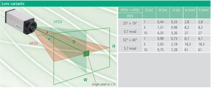
HFOV ... Horizontal Field Of View (horizontal aperature angle)
