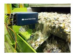
Managing the ash residue is important step for many reasons at incineration facilities around the world. From minimizing the possibility of ash dust inhalation and ingestion of employees, to preventing ash being absorbed into the environment, as well as, to lowering transportation costs due to weight. With MoistTech's NIR Moisture sensor operators will be able to instantly and continuously measure ash moisture and control these problems.
