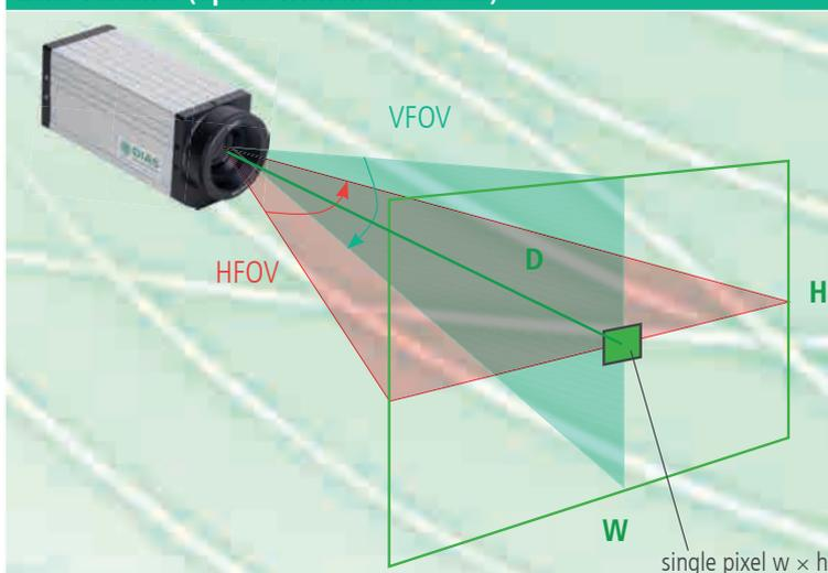
HFOV ... Horizontal Field Of View (horizontal aperture angle)    W ... Image width
