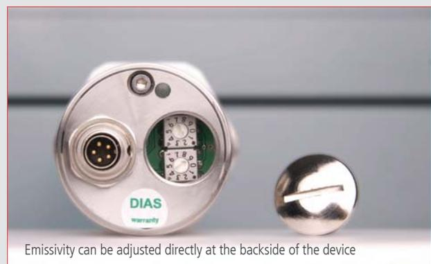
Emissivity can be adjusted directly at the backside of the device
