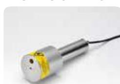
The Laser Sighting Tool screws onto the front of the sensor during installation and indicates precisely where the sensor is aiming. Once the sensor has been aimed at the centre of the target and locked in position the Laser Sighting Tool can be removed. The laser is activated by means of a push button on the front of the tool which has a latching mechanism.
