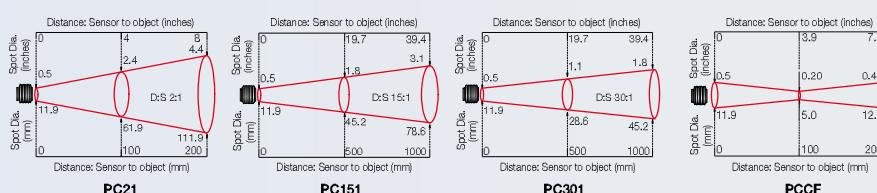
All PyroCouple sensors are fitted with precision Germanium lenses for accurate optics. Model PC21 has 2:1 optics making it suitable for most applications where the sensor can be mounted close to the target. Model PC151 is designed for small or distant targets and has an optical resolution of 15:1. Model PC301 is designed for very small or distant targets and has an optical resolution of 30:1. Model PCCF is designed for targets as small as Ø5mm at a distance of 100mm from the sensor.
