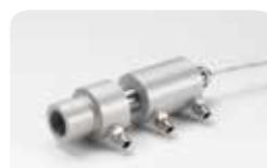
The air/water cooled housing allows the sensor to withstand ambient temperatures which exceed the normal 70°C limit. Air or water (depending on required) flows into one of the fittings on the side and out of the other. To prevent condensation forming on the lens, the air/water cooled housing is supplied complete with an air purge collar. Please note, the air/water cooled housing must be ordered with the sensor and cannot be fitted by the user.
